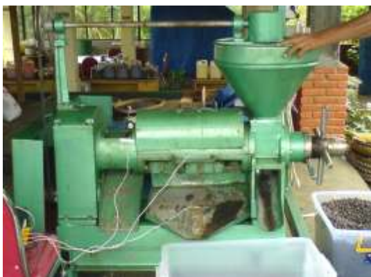
Gambar 2. Mesin pres biji jarak tipe double stage screw expeller (BBP Mektan)
