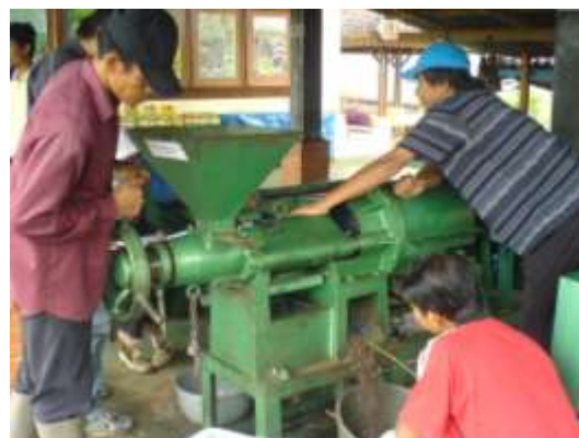
Gambar 3. Mesin pres biji jarak tipe single stage screw expeller (Balitri, Pakuwon)
