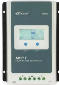
Gambar 3. 2. Solar charger controller
