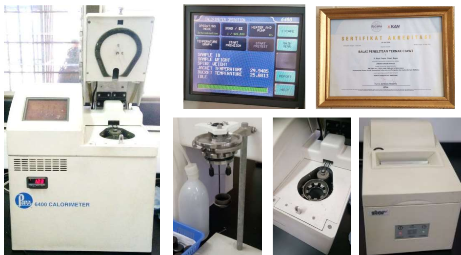
Gambar 3.33. Parr 6400 Bomb Calorimeter
