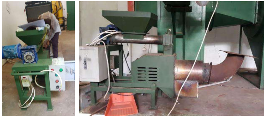
Gambar 3.9. burner , motor burner dan Inverter burner
