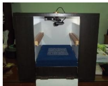
(a) Kotak pengambilan citra beras / (b) Image acquisition chamber
