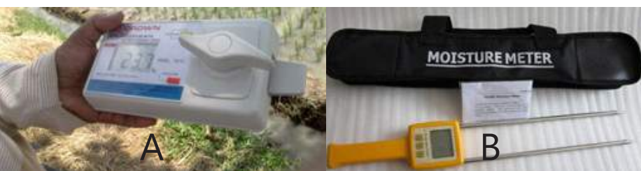
Gambar 3. Alat pengukur kadar air gabah (moisture tester)
