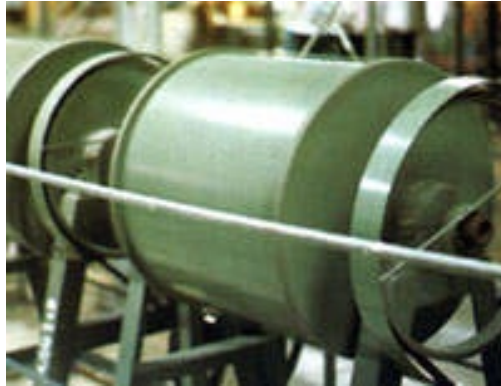
Gambar 38. Alat balls mills Sumber : Murphy (1990)
