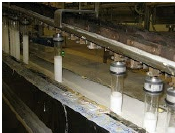
Gambar 41. Proses dipping Sumber : Murphy (1990)
