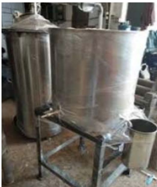
Gambar 1. Alat pirolisis asap cair Figure 1. Pyrolysis pan to produce liquid smoke Sumber/Source : Girard (1992)
