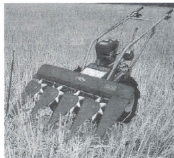
Gambar 8.6. Alat panen reapper 4 row
