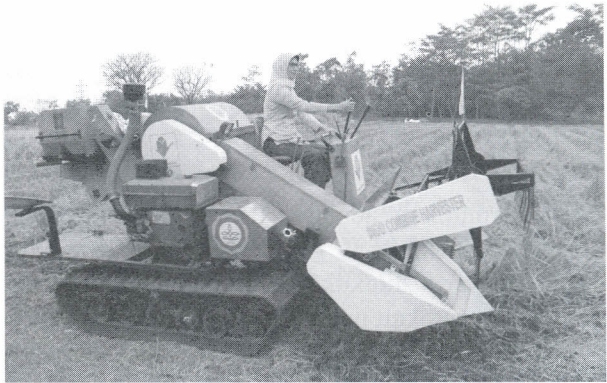
Gambar 8.9. Mesin panen padi riding type (Indo-Combine Harvester)
