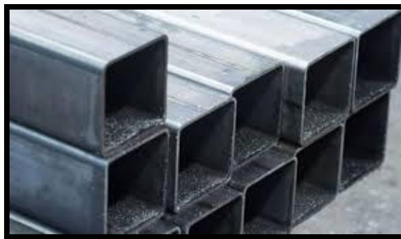
Gambar 2.15 Besi Hollow galvanis (Sumber: https://wira.co.id/besi-hollow )
