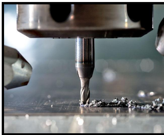
Gambar 2.8 Proses Mesin milling (Sumber: https://kentusa.id/product-categories/milling-machines/ )
