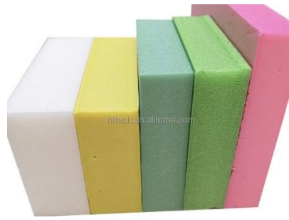
Gambar 4.23. Busa XPS ( extruded polystyrene ) (sumber: https://indonesian.alibaba.com/ )
