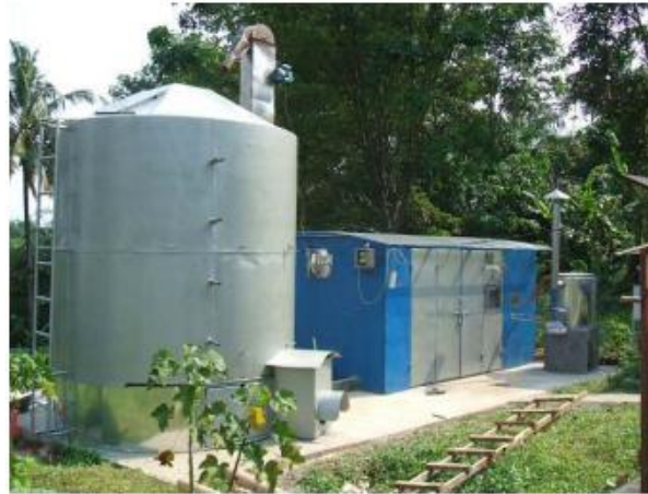
Gambar 2.5. Pengering ERK- hybrid dan ISD terintegrasi (sumber: http://repository.ipb.ac.id/handle/123456789/8259 )
