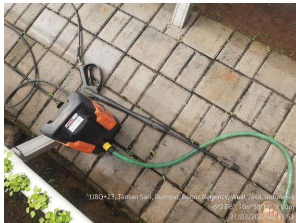
Gambar 4. 6. High Prassure Cleaner tipe ABW VBB 70 (Sumber : Dokumen Pribadi)
