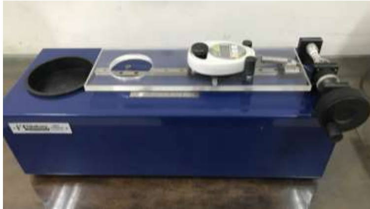
Gambar 6. Surface shear test apparatus
