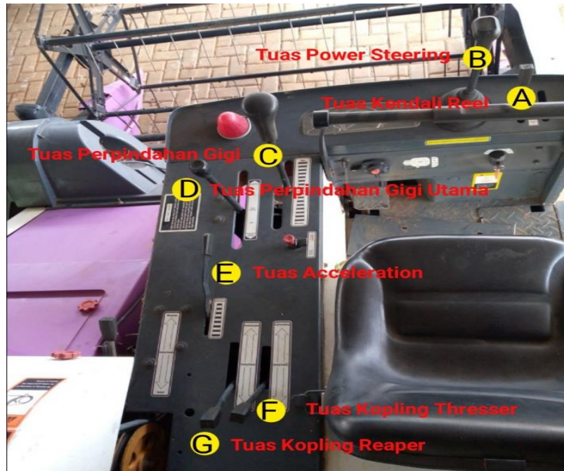
Gambar 2. Tuas pengontrol combine harvester
