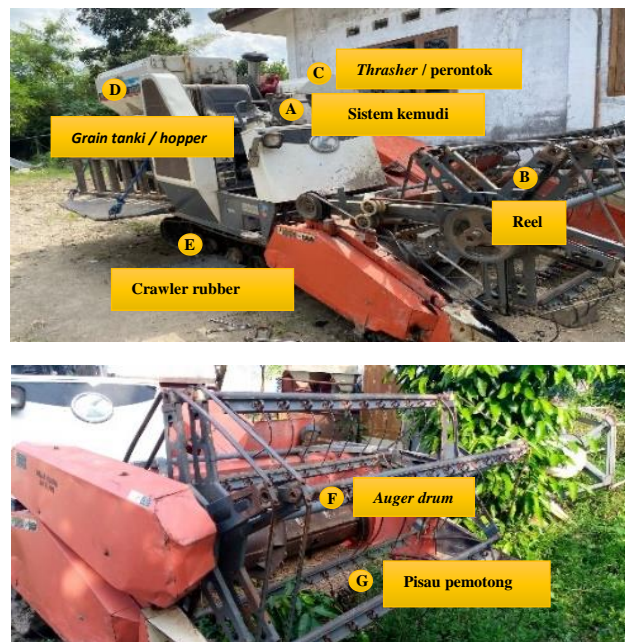
Gambar 11. Bagian-bagian combine harvester Kubota DC-60
