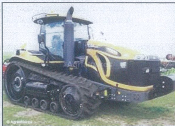
Gambar 63. Traktor roda Track/(Crawler Karet) ( https://www.google.co.id/search?q=traktor , April 2016)
