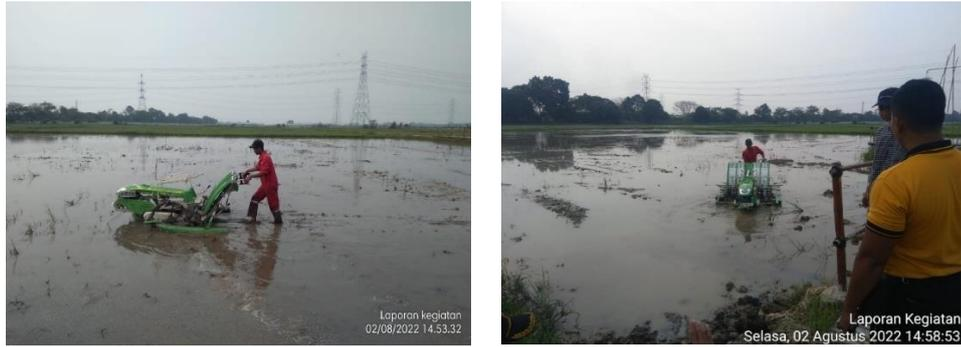
Gambar 4. Pengoperasian mesin *rice transplanter*
