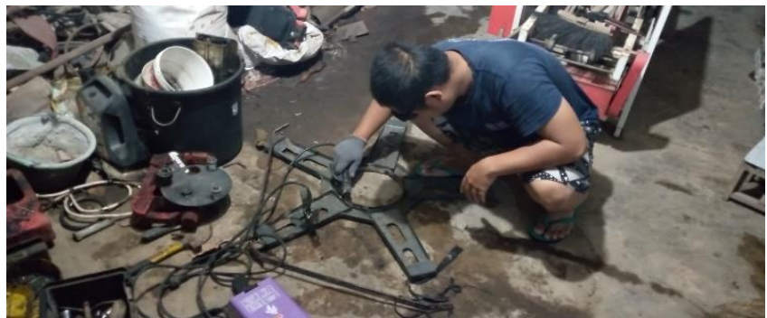
Gambar 4. 19 Mengelas reel combine harvester
