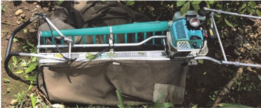
Gambar 1. Mesin pemanen daun teh tipe GT 120 Ochiai Figure 1. The tea leaf harvester type GT 120 Ochiai
