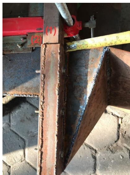
Gambar 4.9. hollow (1), besi L (2)
