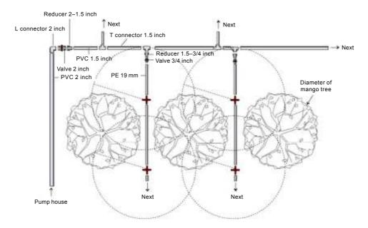
Fig. 2. Fan jet sprayer irrigation technique on mango trees at Cukurgondang Experimental Station, Pasuruan, East Java.
