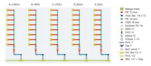
**Fig. 1.** Design of experimental plots of fan jet sprayer irrigation technique on mango trees at Cukurgondang Experimental Station, Pasuruan, East Java.
