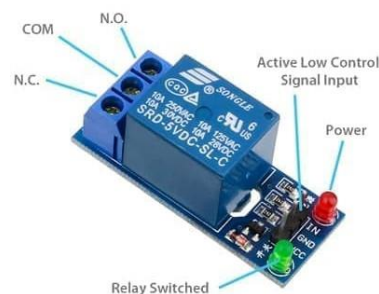
Gambar 2. 4. Relay Module .
