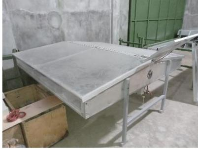
Gambar 4. 19. *Solar Dryer Portable*
