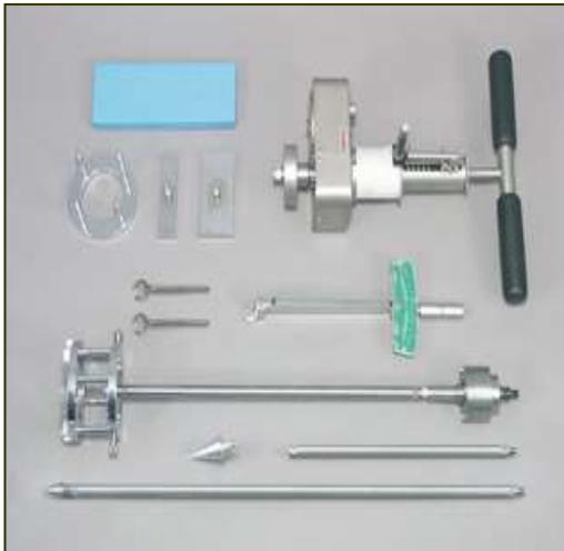
Gambar 2. Alat Penetrometer SR-2
