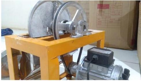
Gambar 6: Transmisi mesin perajang sawut singkong.
