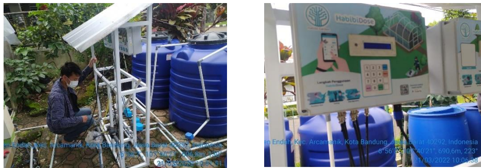
Gambar 8. Control panel Pecampuran Pupuk AB Mix
