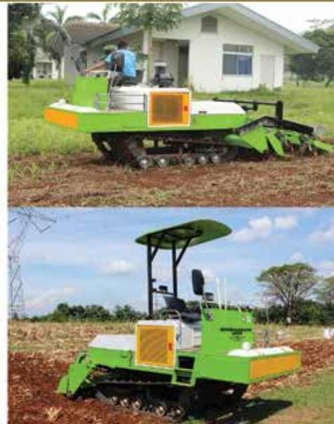
*Land Preparation and Integrated Grain Cultivation or Rota Planting Machine is able to save time and energy in cultivation and planting activities conducted in one process activity. This machine has a driving source in the form of diesel engine, equipped with a liquid fertilizer applicator that serves to spray the granules of liquid fertilizer to soil and plants.*
