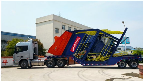
Gambar 11. Mesin AMP yang bergerak Sumber : Sinosun Machinery (2018) Figure 11. AMP mobile machine Source: Sinosun Machinery (2018)
