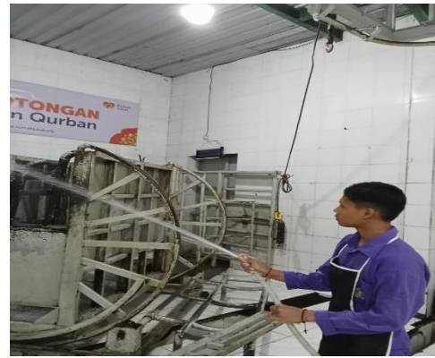
Pembersihan restraining box
