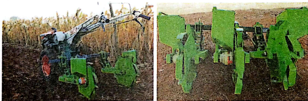
Gambar 4. Alat tanam suntik bergulir ( Rolling Injection Seeder )
