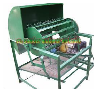
Gambar 3. Silinder Perontok Padi (sumber makmurmekanik 2014)
