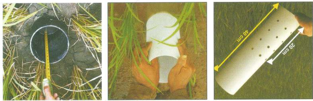
Figure 4. Left is a PVC pipe, center is the practice how to embed water pipe into the soil, and right is how to measure water depth using water pipe
