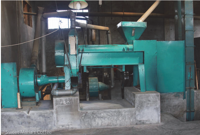
Gambar 14. Mesin Giling Basah ( Huller HS basah ) [Sumber: Sweet Maria's Coffee]
