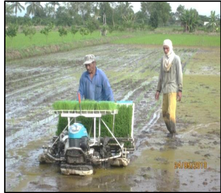
Gambar 20. Alat Tanam Mekanis (Rice Transplanter)
