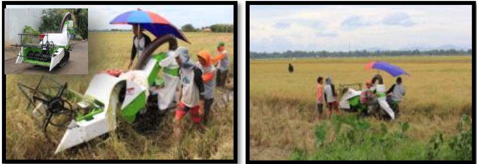
Gambar 10. Pengujian mesin panen padi tipe combine harvester prototipe II
