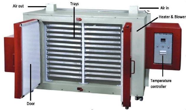
Gambar 2.2 Cabinet dryer (Nayak et al. , 2018)
