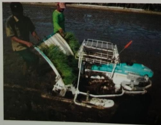
Gambar 8. Penerapan alat tanam ( rice transplanter ) di lahan pasang surut
