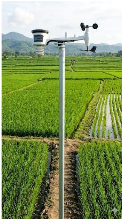
Gambar 7. Automatic Weather Station
