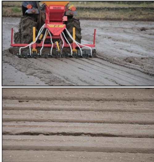
Gambar 2. Alat tanam benih drum seeder dan mesin direct seeding
