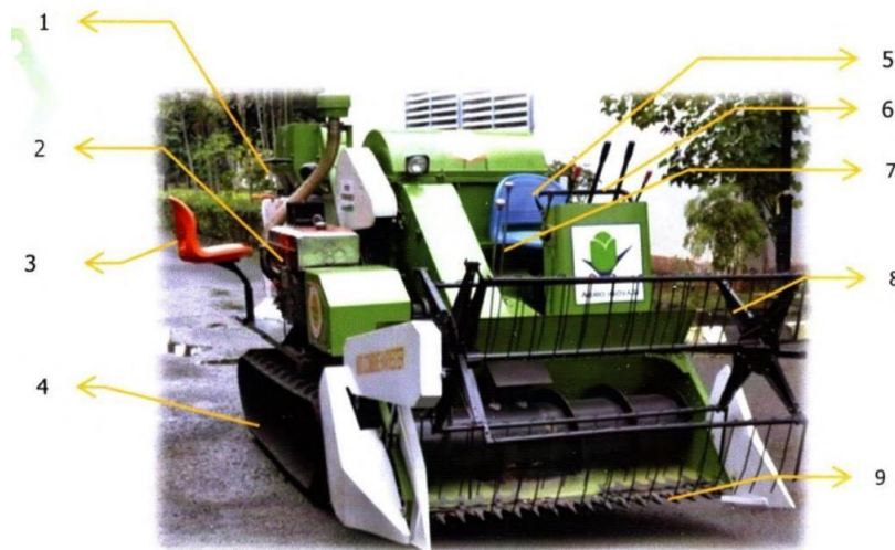
Gambar 2. 1. Bagian – bagian mesin combine harvester (1) grain output (2) Bagian mesin/engine (4) rubber track (6) tuas kendali (7) tuas persneling (8) header unit (9) cutter bar
