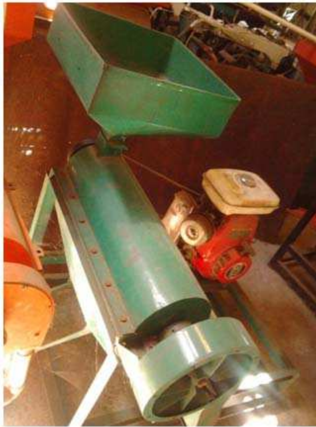
Gambar 6. Mesin sosoh sorgum tipe abrasif Balai Penelitian Tanaman Sereal
