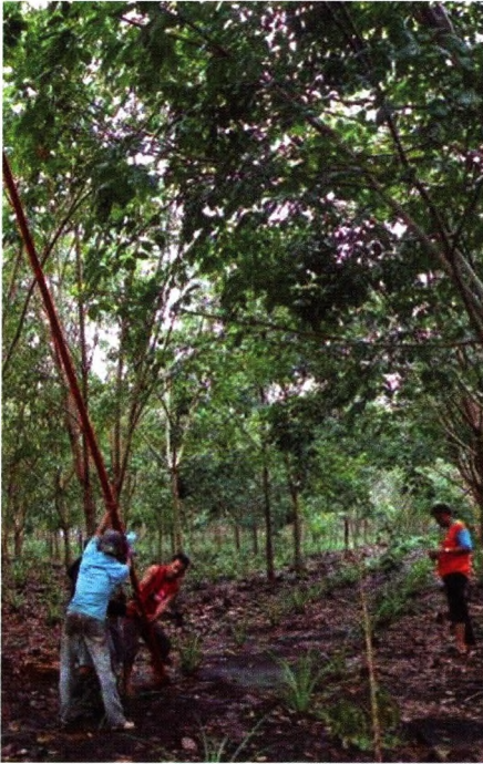
Gambar 36. Penelitian subsiden gambut, menanam pipa besi 8-12 m di 6 lokasi (5 April 2012).
