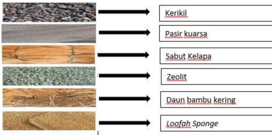
Gambar 3. 3. Susunan media filter air
