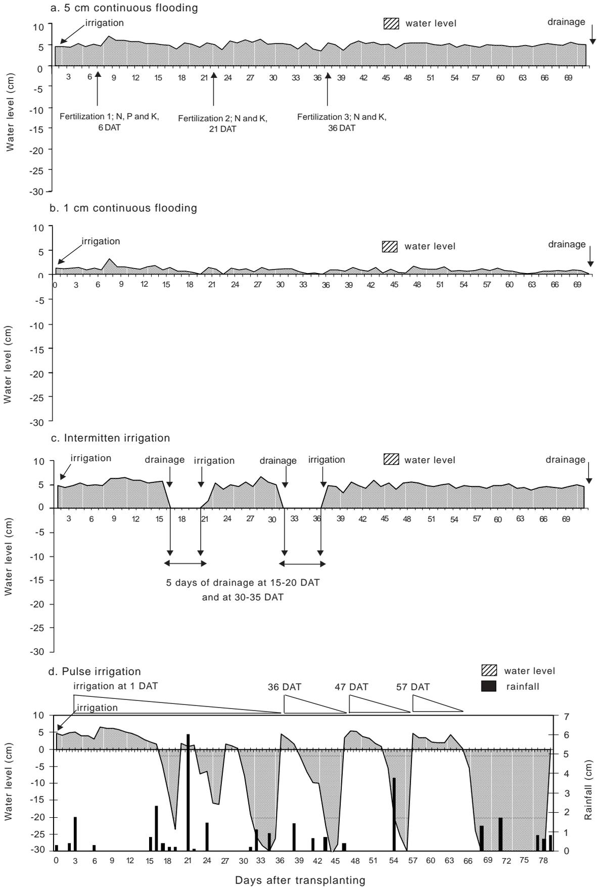
**Fig. 4.** The water level in the experimental plots treated under four different water regimes and the daily rainfall amount (Figure 4d, in bars), Jakenan Experimental Farm, Central Java, dry season of 2002.
