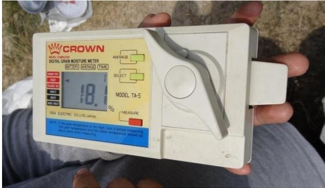
Gambar 2. Moisture tester pengukur kadar air gabah
