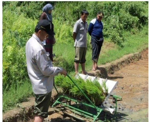
Gambar 2. Pengoperasian alat penanam
