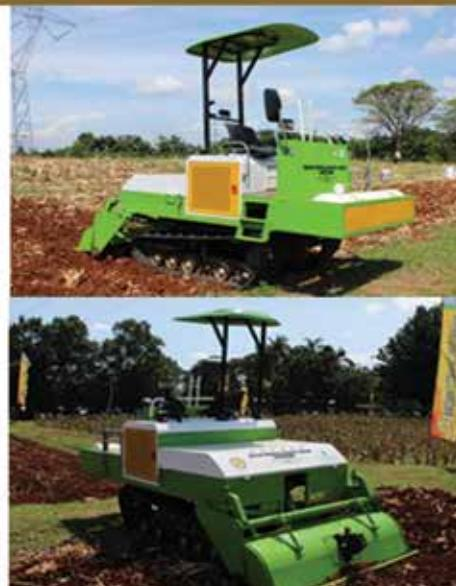
*This machine is engine by a 60 PK diesel motor, using rotary plow implements with rubber crawler wheels, which can be used for both wet and dry soil areas, saving time, fuel and labor. This machine serves to till the soil as well as to chop the remaining rice straw, corn crop, and weeds and mix with soil, to increase the content of soil organic matter. This machine is also equipped with decomposer sprayers to accelerate the process of bio-decomposition.*
